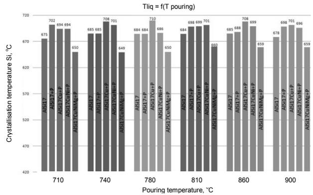
Fig. 3. Changes of temperature  $T_{liq}$  as a function of pouring temperature
