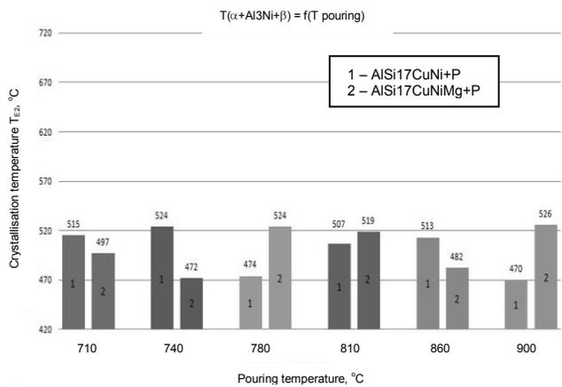
Fig. 7. Changes of temperature  $T_{E2}$  (the Ni containing eutectic) as a function of pouring temperature
