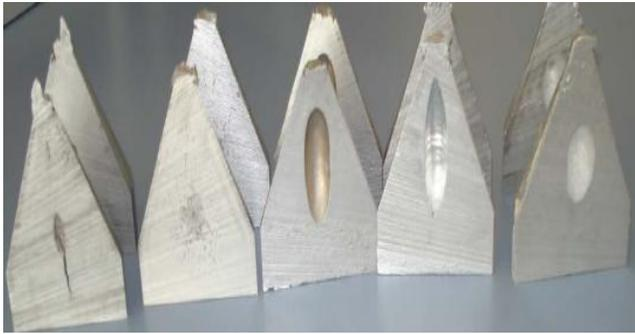
Fig. 3. Typical shrinkage porosity obtained using Tatur test
