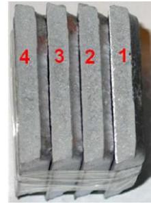
Fig. 5. Fractured pieces of K-mold test sample
