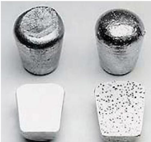
Fig. 1. Test samples (A) solidified under atmospheric pressure and (B) solidified under vacuum
