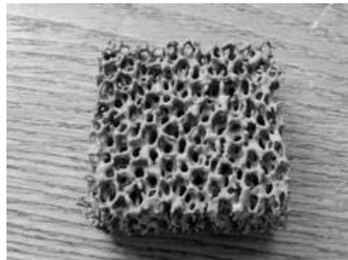
Fig. 2. Filter after the application of inoculating layers
