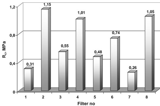
Fig. 4. Compression strength compared for different filters
