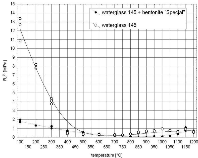
Fig. 1. Effect of baking temperature on residual strength of microwave-hardened moulding sand containing bentonite addition
