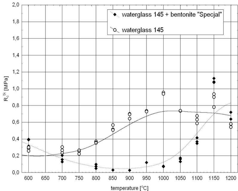
Fig. 2. Effect of baking temperature on residual strength of microwave-hardened moulding sand containing bentonite addition
