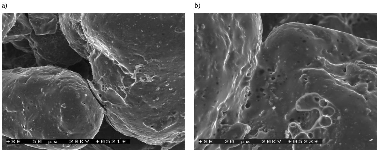
Fig. 6. Linking bridges in moulding sand with waterglass 145 and with bentonite addition after baking at 950 °C: a) adhesive-type destruction of linking bridges, b) surface and internal structure of a linking bridge
