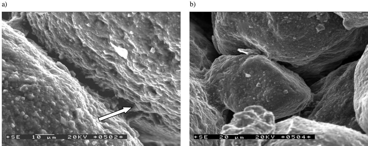
Fig. 3. Linking bridges in moulding sand with waterglass 145 and with bentonite addition, after baking at 100 °C: a) crack of an adhesive-type bridge, indicated by the arrow, b) complex of bridges
