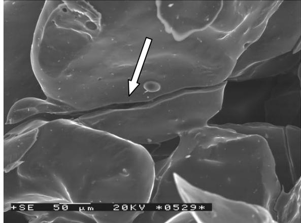
Fig. 7. Linking bridges in moulding sand with waterglass 145 and with bentonite addition after baking at 1200 °C:
