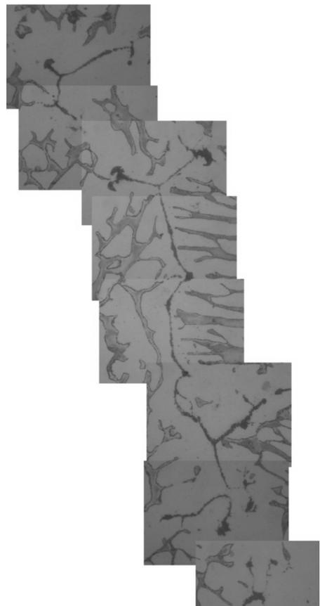
Fig. 4. A hot crack in the cast steel No. 4 containing 0,08% C and 2,62% Cu, magnification 100x
