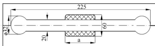
Fig. 1. A scheme of the die for testing the hot cracking susceptibility
