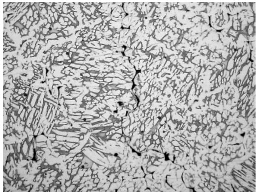
Fig. 3. The crack trajectories in specimens a) cast steel containing C=0,02%; with Cu b) cast steel containing C=0,02%; without Cu, magnification 100x
