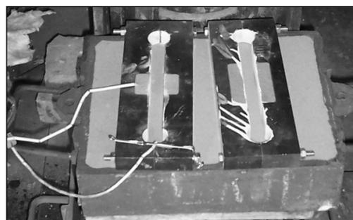
Fig. 2. Metal moulds for testing of hot cracking susceptibility directly after pouring
