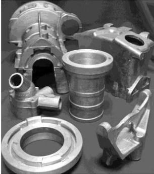
Fig. 1. Examples of aluminum castings
