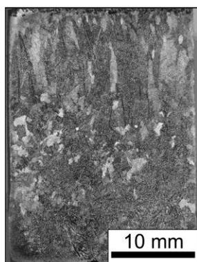
Fig. 1. Macrostructure of the examined casting wall
