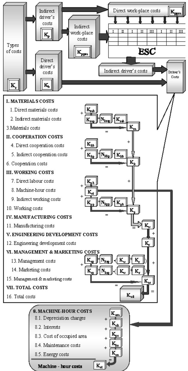
Fig. 4. Own cost estimation with the method of additional calculation according to cost centres
