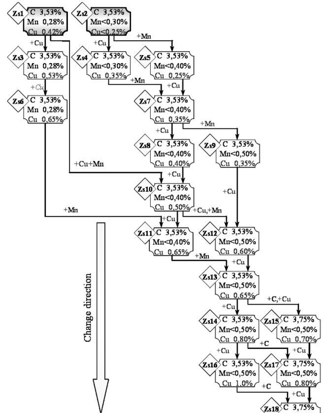
Fig. 2. Planning of pouring order depending on spheroidal graphite iron composition
