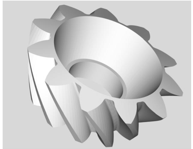
Fig. 3. CAD model of gear with a relief
