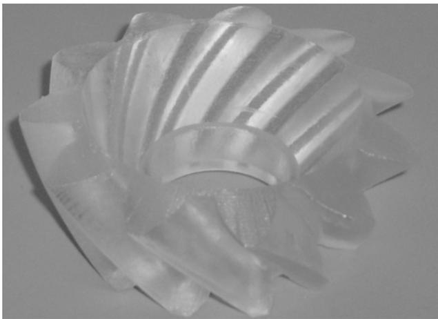
Fig. 6. SLA model of gear
