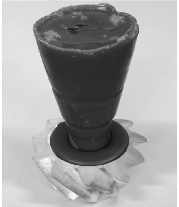
Fig. 7. Hybrid pattern of gear with gating system
