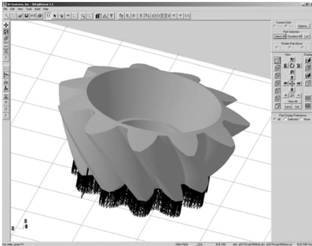
Fig. 5. Model on work platform (3D Lightyear software)
