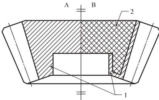
Fig. 2. Cross sections of analyzed gear: A – full pattern, B – hybrid pattern; 1 – resin, 2 – casting wax
