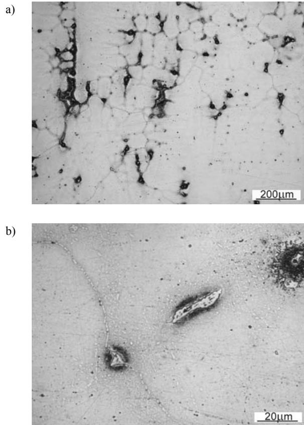
Fig. 3. Microstructure of the investigated cast steel after the solution heat treatment from 1080 °C and aging at 600 °C. Vickers hardness 176. a) morphology of interdendritic precipitates; b) precipitations in grain boundaries
