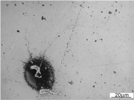
Fig. 4. Microstructure of the investigated cast steel after the solution heat treatment from 1150 °C. Vickers hardness 195
