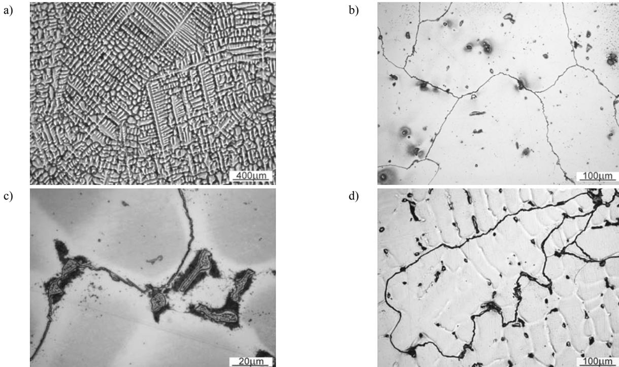
Fig. 1. Microstructures of the investigated cast steel in as-cast condition a) dendritic structure revealed by an intensive etching; b) continuous network of precipitates in grain boundaries; c) precipitates in interdendritic areas; d) localisation of precipitates in relation to dendritic structure. Vickers hardness 204
