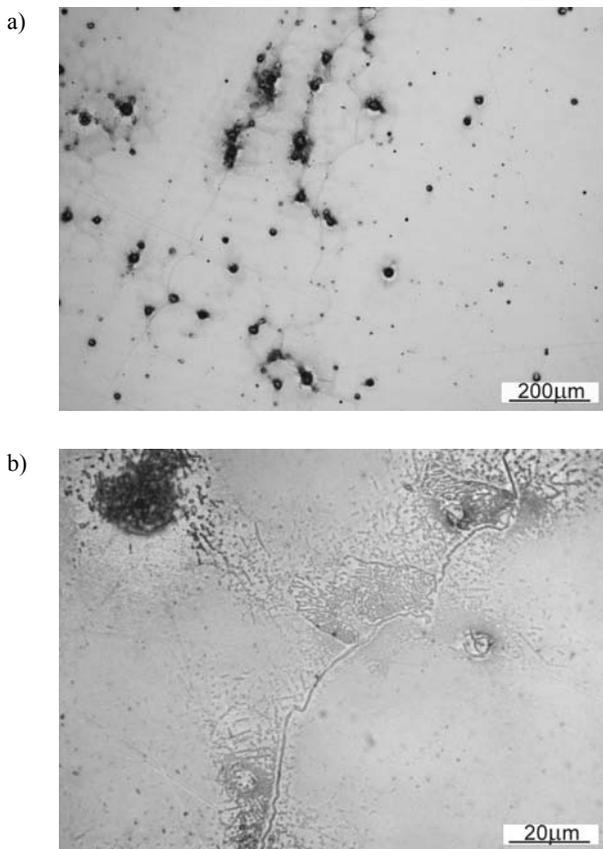
Fig. 2. Microstructure of the investigated cast steel after the solution heat treatment from 1080 °C. Vickers hardness 205. a) morphology of interdendritic precipitates, b) precipitates in grain boundaries
