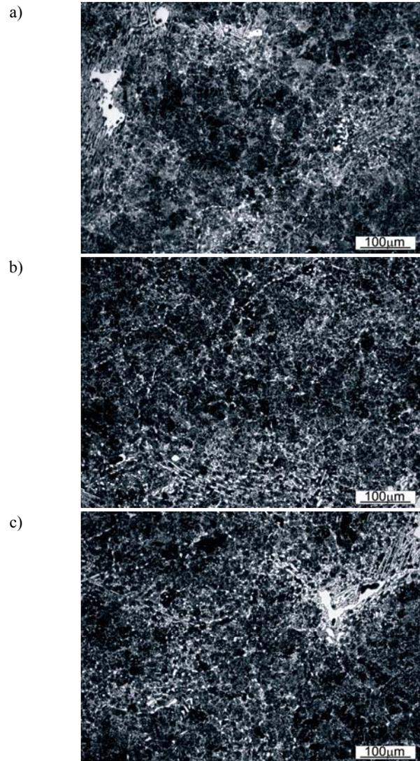
Fig. 2. Microstructure of G155CrNiMo4-3-3 cast steel after the heat treatment: a) short variant; b) medium variant; c) long variant. Etched with 2 % nital
