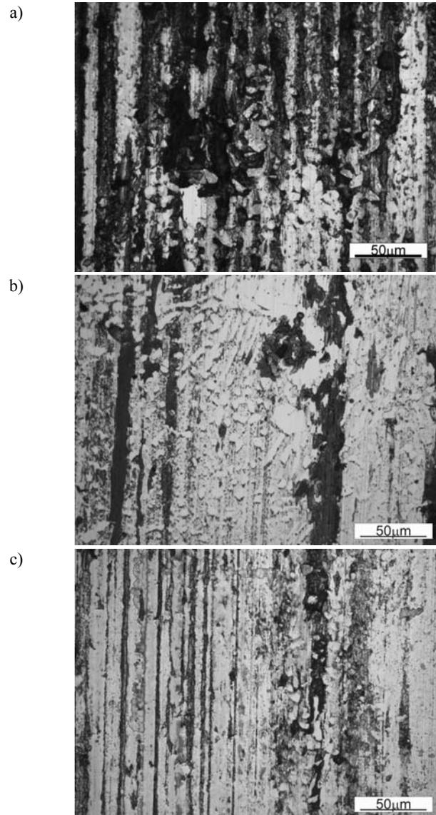
Fig. 6. Tribologically worn surface of the cast steel sample after the long variant of the heat treatment: a) load: 50 N, b) load: 100 N, c) load: 150 N
