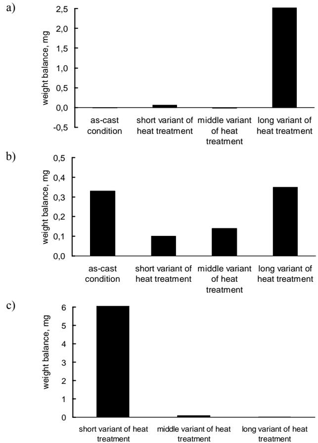
Fig. 7. Weight balance for samples after tribological testing: a) under a load of 50 N, b) under a load of 100 N, c) under a load of 150 N
