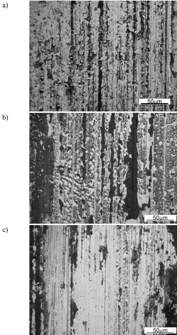
Fig. 5. Tribologically worn surface of the cast steel sample after the medium variant of the heat treatment: a) load: 50 N, b) load: 100 N, c) load: 150 N
