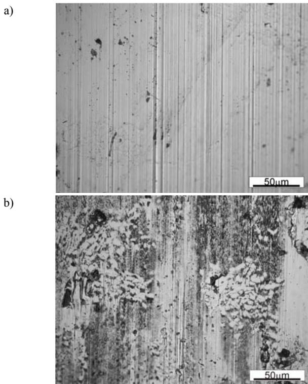
Fig. 3. Tribologically worn surface of a cast steel sample in as-cast condition: a) load: 50 N, b) load: 100 N
