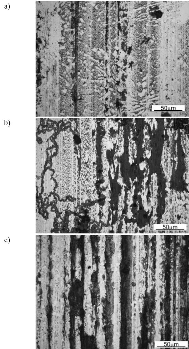
Fig. 4. Tribologically worn surface of a cast steel sample after a short variant of the heat treatment: a) load: 50 N, b) load: 100 N, c) load: 150 N
