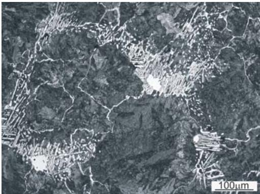
Fig. 1. Microstructure of G155CrNiMo4-3-3 cast steel in as-cast condition. Etched with 2% nital
