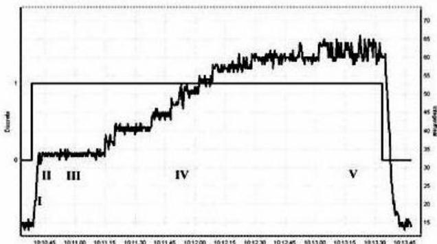
Fig. 3. Power consumption by the drive in the mixing system of a turbine mixer MTP-500: I- charging of mix components; II- homogenisation; III- water dosing; IV- mixing of wet sand; V- emptying the mixer
