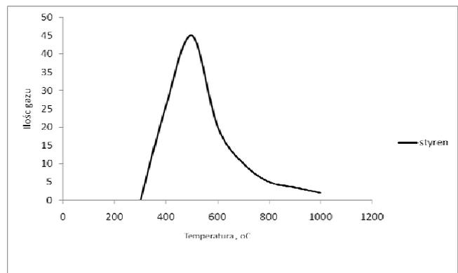
Fig. 3. Styrene volume [µg/g] formed in function of temperature T °C
