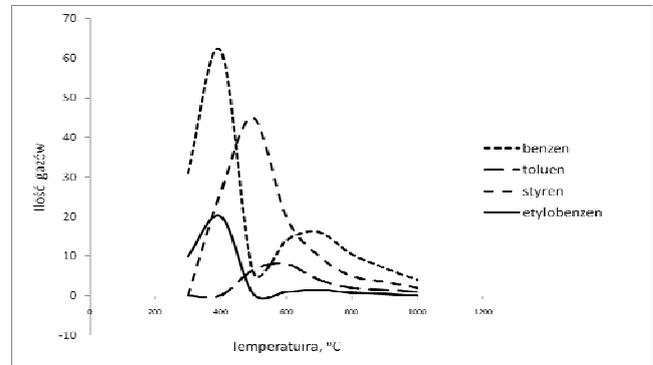
Fig. 1. Gas volume [µg/g] emitted in function of temperature T °C
