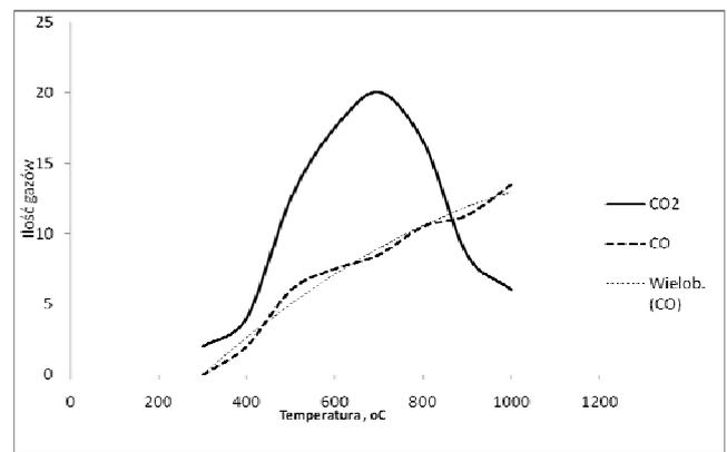
Fig. 2. Gas volume [µg/g] emitted in function of temperature T °C
