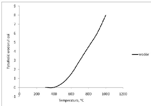
Fig. 4. Hydrogen volume [ $\mu\text{g/g}$ ] emitted in function of temperature T  $^{\circ}\text{C}$
