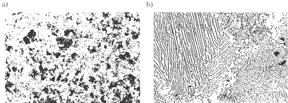
Fig. 2. Microstructure of the GA8 alloy in T4 condition, a) magn.100x, b) magn.500x
