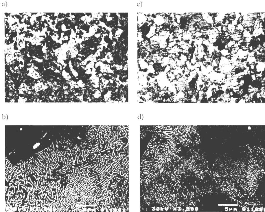
Fig. 4. Microstructure of the GA8 alloy in T6 condition;
