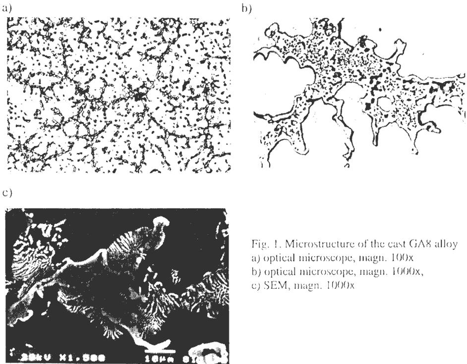
Fig. 1. Microstructure of the cast GA8 alloy
