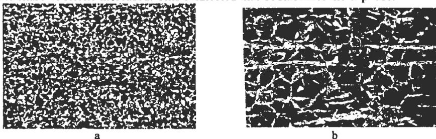
Figure 2. The metal microstructure of tubular billet from microalloying (a) and compared (b) steels (magnification 50x).
