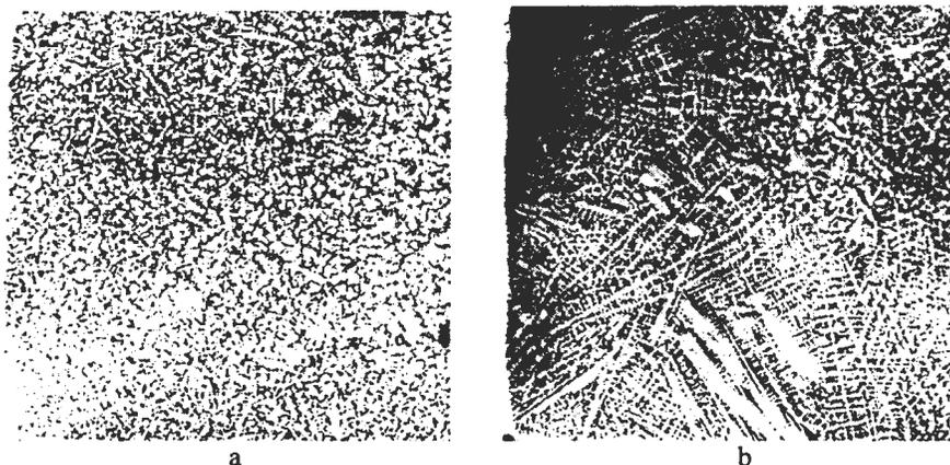
Figure 1. Fragment of macrostructures of middle carbon steel ingots (0.002 t) with addition 0.04 %Ti) (a) and without microalloying (b) (magnification 6x).
