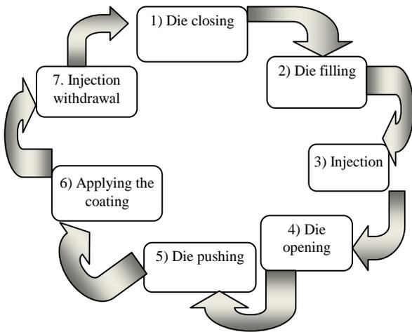
Fig. 1. Die casting cycle in IDRA 7000
