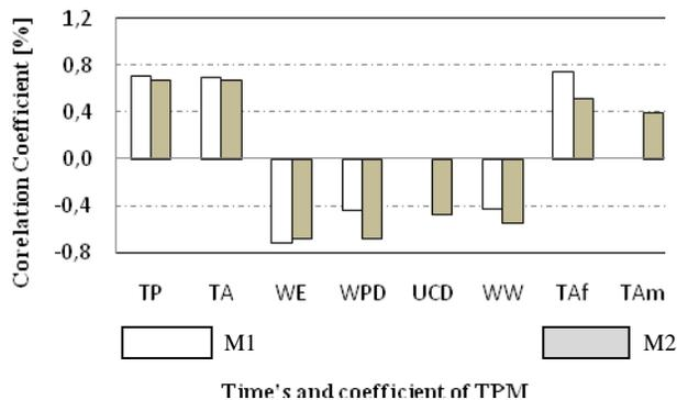
Fig. 5. Comparison of the effect of TPM factors in both studied machines
