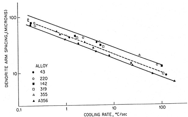
Fig. 2. The effect of average cooling rate on the size of dendrite arm spacing for six aluminium alloys [1]. The data cover a range of cooling rates of three order of magnitude
