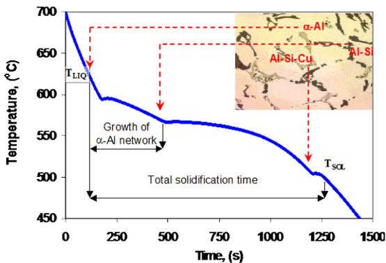
Fig. 1. The cooling curve of AlSiCu alloy with schematically designated areas of typically precipitated phases
