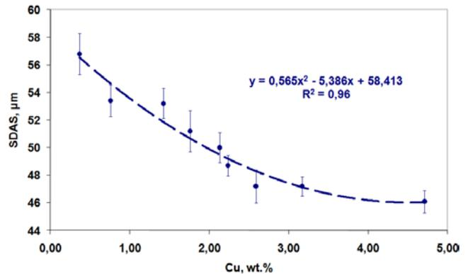
Fig. 5. The effect of the various copper contents on the size of the SDAS. The increases in the copper content from 0 to 3 weight percent refine considerably the size of the SDAS
