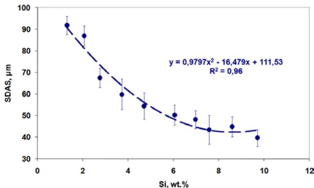
Fig. 4. The effect of the various silicon contents on the size of the SDAS. There is appreciable refining effect as the content of silicon varied between 1 and 8 weight percent
