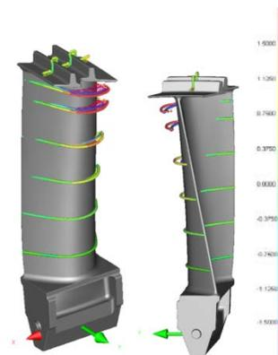
Fig. 3. Measured dimensions differences shown on 3D model
