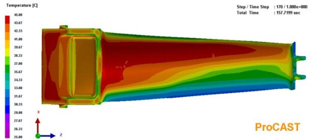
Fig. 7. Wax blade just removed from mould, simulation
