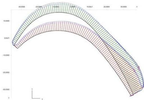
Fig. 8. Measured deformations of wax pattern at  $z=160\text{mm}$
