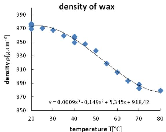
Fig. 4. Density of model wax related to temperature
