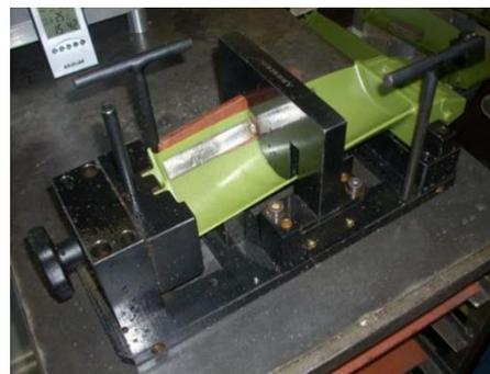
Fig. 1. Wax model of blade fixed in jig
