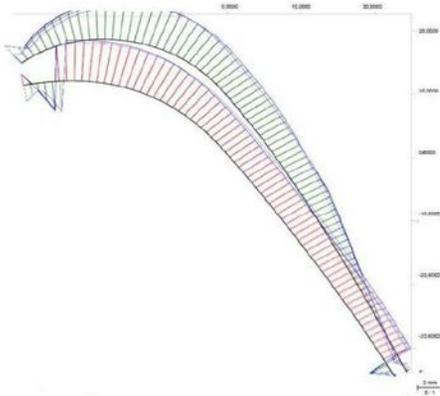
Fig. 9. Measured deformations of casting at  $z=265\text{mm}$
