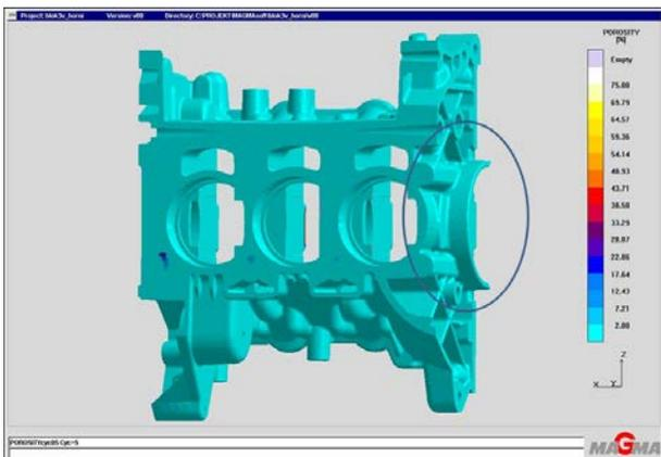
Fig. 13. Porosity measured in 4<sup>th</sup>-bearing area of engine block, die-cast with LSC, top view of bearing [6]
