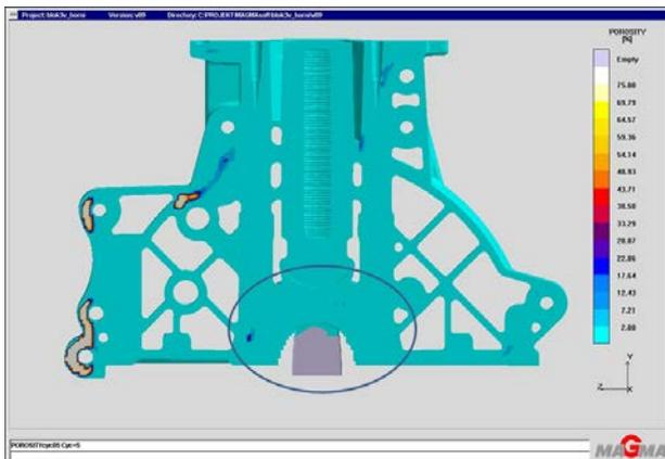
Fig. 12. Porosity measured in 4<sup>th</sup>-bearing area of engine block, die-cast without LSC, lateral view [6]
