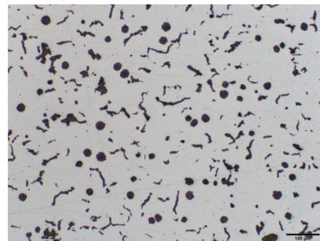
Wall thickness 8mm, 0.013%Mg, 24.9%SGI
