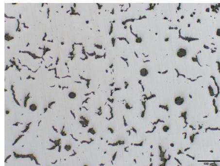
Wall thickness 16mm, 0.013%Mg, 15.2%SGI
