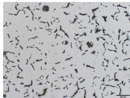
Wall thickness 40mm, 0.013%Mg, 1.5%SGI
