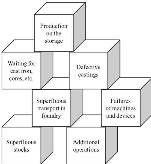
Fig. 1. Areas of wastage in a foundry
