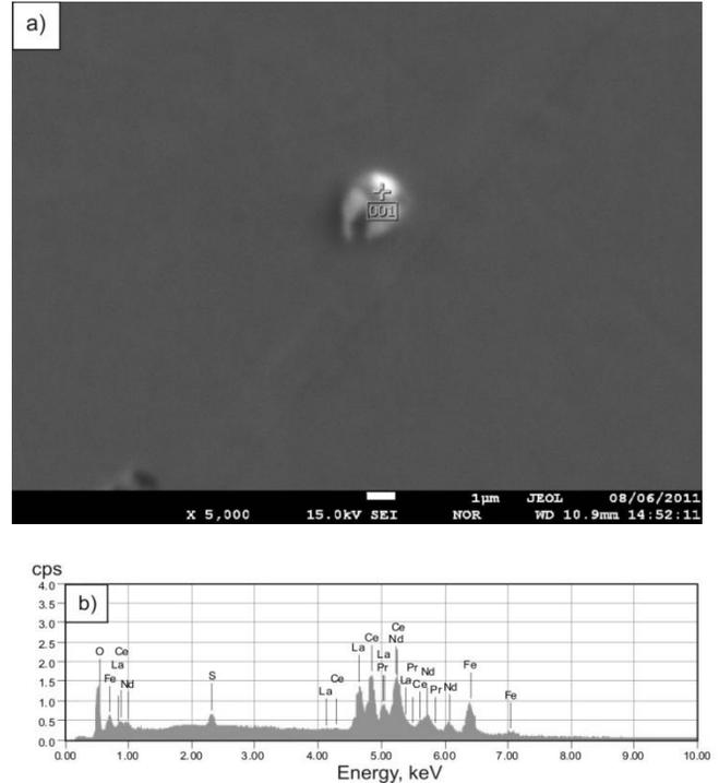
Fig. 4. Oxysulfide type non-metallic inclusion modified with rare earth elements: a – view of the inclusion, b – spectrum of the inclusion (steel B after forging)
