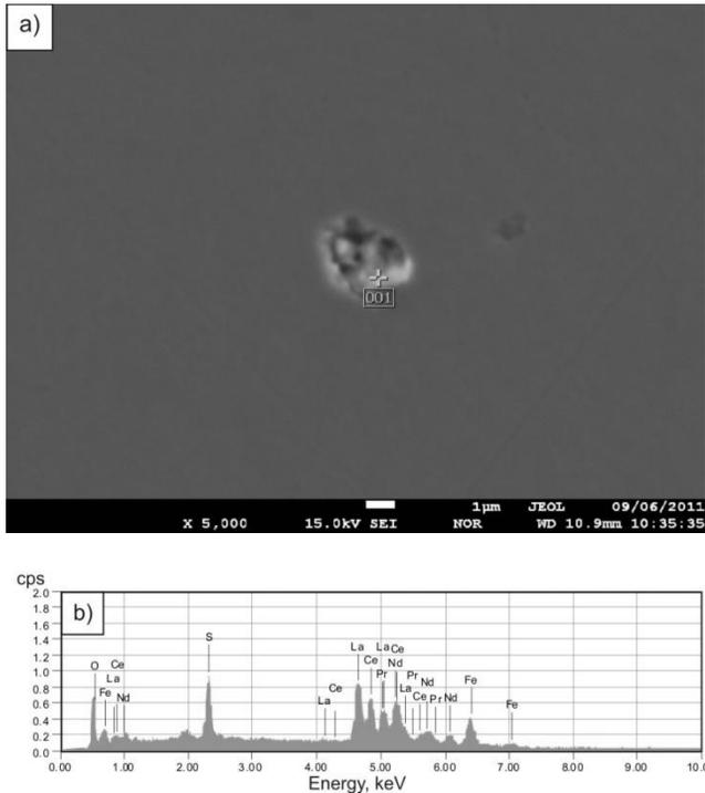
Fig. 3. Oxysulfide type non-metallic inclusion modified with rare earth elements: a – view of the inclusion, b – spectrum of the inclusion (steel A after forging)
