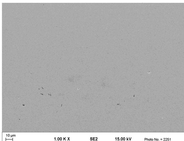
Fig. 2. Very fine non-metallic inclusions on the longitudinal section of the B steel sample
