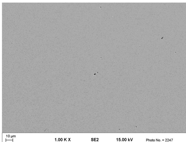
Fig. 1. Very fine non-metallic inclusions on the longitudinal section of the A steel sample
