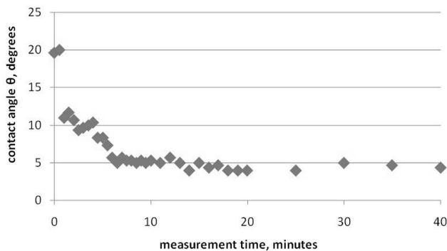
Fig. 6. Time-related changes in the value of contact angle in a quartz-modified water glass system (5wt.% suspension of ZnO nanoparticles in propanol). Measurement temperature: 20°C
