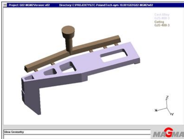
Fig. 1. The technology of making the casting of a base
