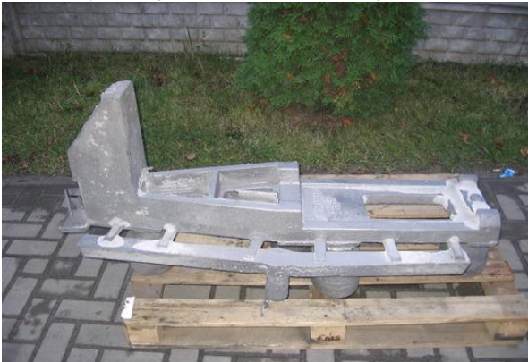
Fig. 4. Casting of the base weighing 102 kg. GJS 400-15
