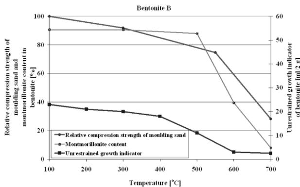
Fig. 3. Results of the unrestrained growth indicator, montmorillonite content and compression strength in dependence of the holding temperature – for bentonite B.
