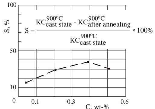
Fig. 3. Effect of carbon content and annealing process on the value of S parameter determined for cast steel of the 17%Cr-36%Ni type [11]. Key to symbols:  $KC_{\text{as-cast state}}^{900^{\circ}\text{C}}$  – the impact resistance of specimen cast at 900°C,  $KC_{\text{after annealing}}^{900^{\circ}\text{C}}$  – the impact resistance of specimen annealed at 900°C/ 400 hours
