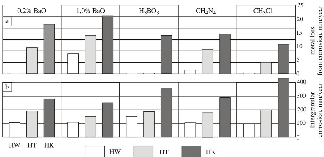
Fig. 6. Corrosion rates in terms of metal loss (a) and intergranular attack (b) observed for three commercial cast alloys in a 20NaCl-25KCl-55BaCl<sub>2</sub> salt bath under different conditions of rectification at 850°C [8]\*; cast steel designations as in Table 1
