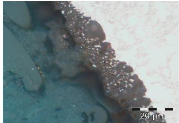
Fig. 1. Anodised layer on the AlSi9Cu4 alloy
