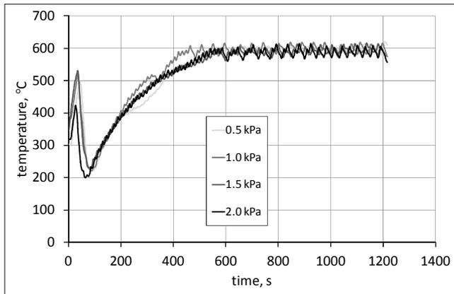
Fig. 7. Temperature in the middle part of the thermal reclaiming chamber in dependence on the set temperature and the air pressure applied for mixing
