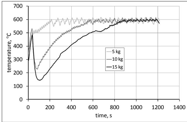
Fig. 11. Temperature pathways in the middle part of the thermal reclaim chamber in dependence on the number of operating burners
