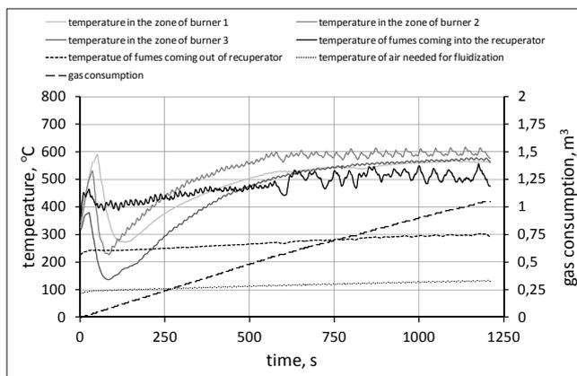
Fig. 4. Temperature values in the selected structural points of the thermal reclaimer
