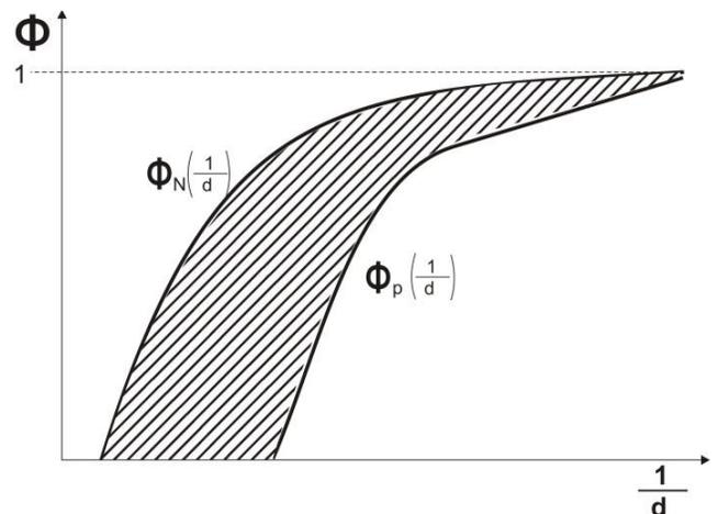
Fig. 5. Interpretation of the work used for the fragmentation of the feed of a diameter  $d_N$  to the product of a diameter  $d_p$  - according to the Rittinger's theory [5]
