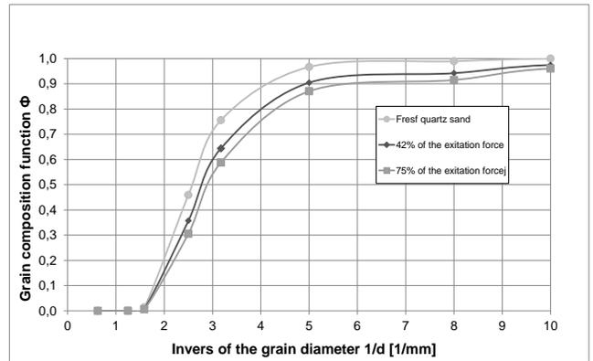
Fig. 10. Grain composition function, at a frequency of 60 Hz and the reclamation time equal 15 min.
