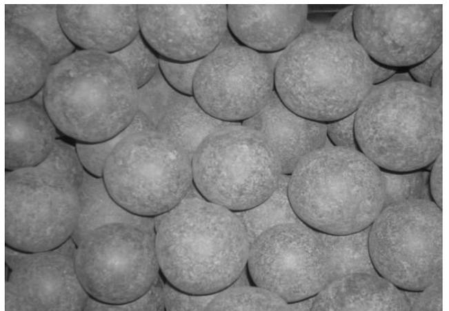
Fig. 3. Cast iron balls, additional grinding-crushing elements of the prototype reclaimer.
