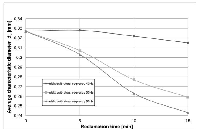
Fig. 7. Changes of the average characteristic diameter  $d_L$  as a function of the reclamation time at three frequencies: 40 Hz, 50 Hz, 60 Hz of electrovibrators operation and the setting of unbalanced masses corresponding to 75% of the maximal excitation force
