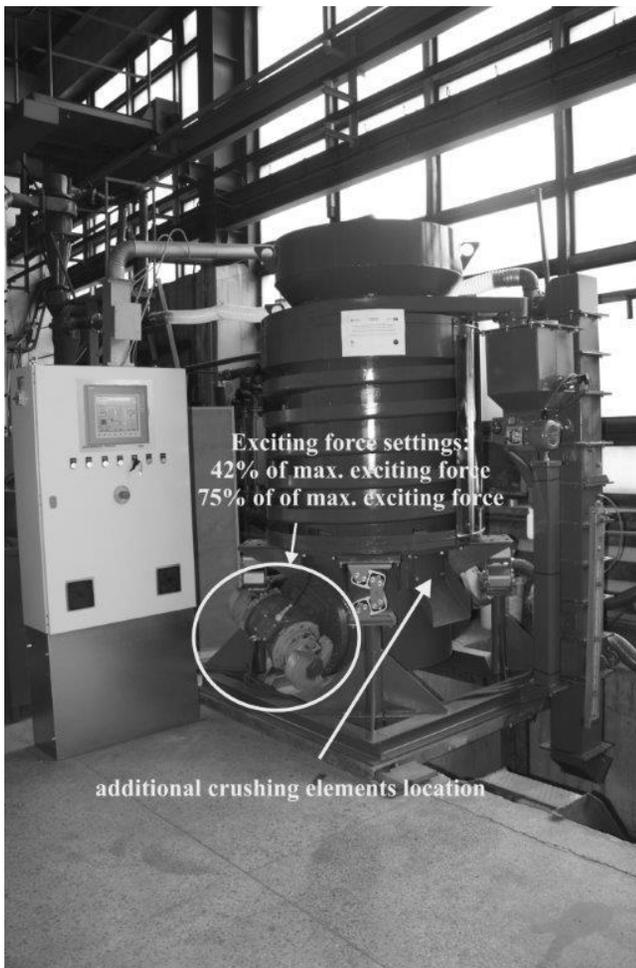
Fig. 1. Prototype vibratory REGMAS reclaimer.
