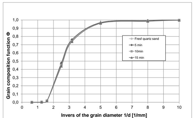
Fig. 11. Grain composition function at 75% of the maximal excitation force and a frequency of 40 Hz for the individual reclamation times
