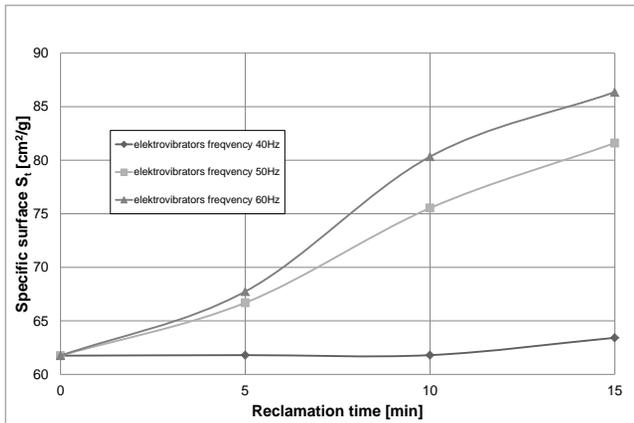
Fig. 8. Changes of the specific surface  $S_t$  as a function of the reclamation time at three frequencies of electrovibrators operations (40 Hz, 50 Hz, 60 Hz) and the setting of unbalanced masses corresponding to 42% of the maximal excitation force
