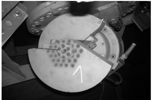
Fig. 2. Example of mutual positioning of flywheels (unbalanced masses) of the electrovibrator.
