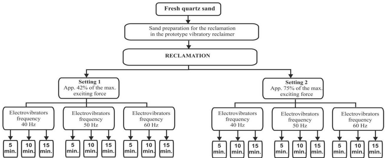
Fig. 4. Schematic presentation of the performed tests
