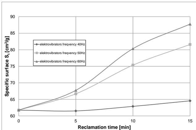
Fig. 9. Changes of the specific surface  $S_t$  as a function of the reclamation time at three frequencies of electrovibrators operations (40 Hz, 50 Hz, 60 Hz) and the setting of unbalanced masses corresponding to 75% of the maximal excitation force
