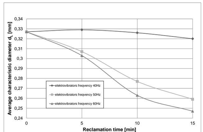
Fig. 6. Changes of the average characteristic diameter  $d_L$  as a function of the reclamation time at three frequencies: 40 Hz, 50 Hz, 60 Hz of electrovibrators operations and the setting of unbalanced masses corresponding to 42% of the maximal excitation force
