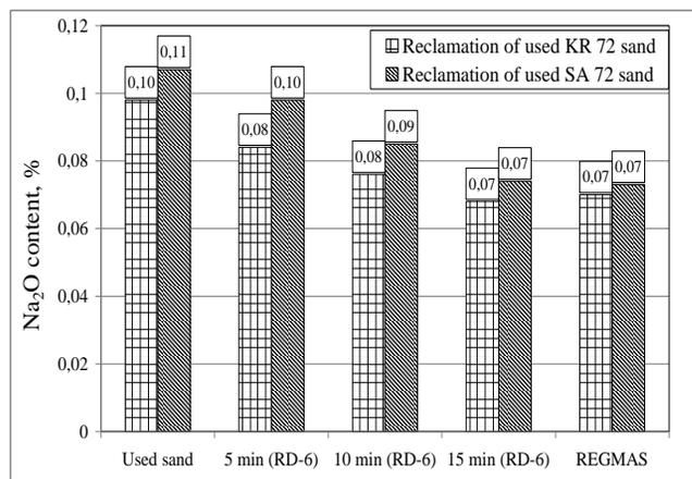
Fig. 6. Na<sub>2</sub>O content on the surface grains of reclaims
