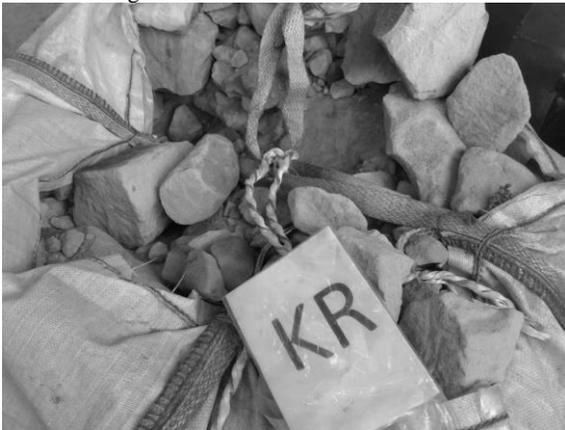
Fig. 1. Spent KR 72 sand before the reclamation process
