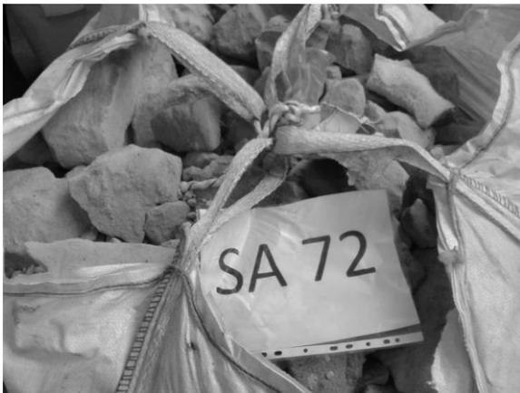
Fig. 2. Spent SA 72 sand before the reclamation process
