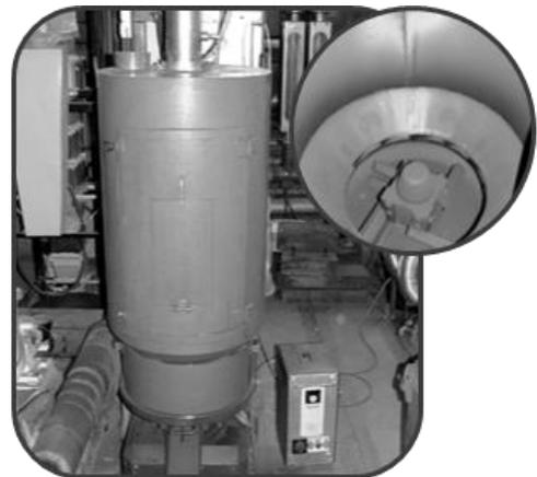
Fig. 4. View of the experimental mechanical rotor RD-6 reclaimer [5]
