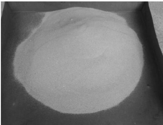
Fig. 3. Spent sand after the preliminary crushing process
