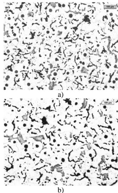
Fig. 2. Microstructure of cast iron in castings with wall thicknesses of (a) 3 mm (using LDASC sand) and (b) 13 mm (using silica sand). Nital etched samples.
