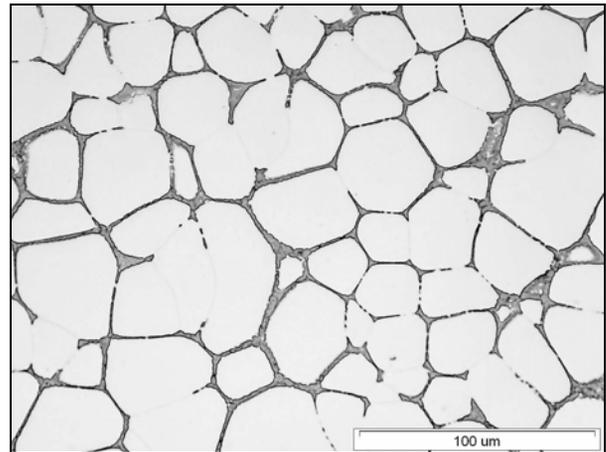
Fig. 1. Optical micrograph of as-cast ZRE1 alloy.
