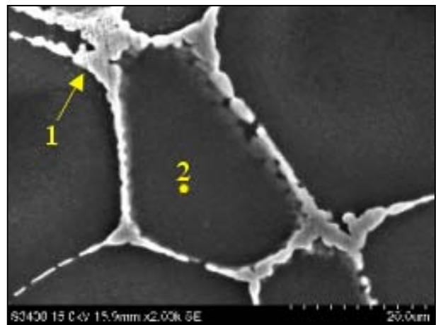
Fig. 2. SEM micrograph of as-cast ZRE1 alloy with marked points of chemical analysis
