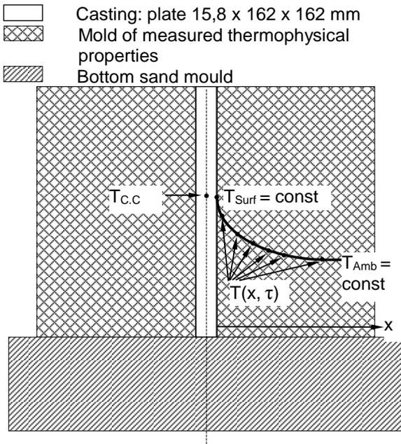
Fig. 1. Scheme of measuring system. Thermocouples location:  $T_{C.C}$  – centre of the casting;  $T_{\text{Surf}}$  – surface of sand mould;  $T(x, \tau)$  – thermocouples located in different distances from the surface;  $T_{\text{Amb}}$  – mould temperature unchanged during the solidification of casting (ambient temperature for the casting)
