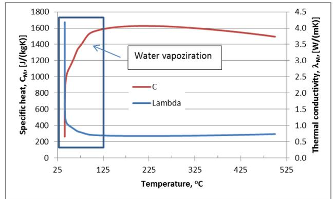
Fig. 5. The Relationships: thermal conductivity vs. temperature obtained in the *Casting Method* experiment for the examined green-sand
