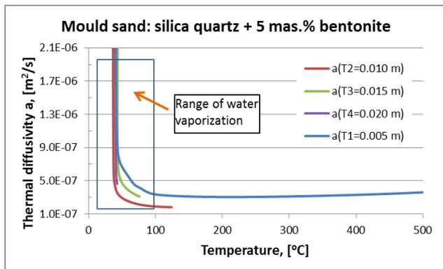
Fig. 4. The thermal diffusivity coefficient calculated from the registered temperature field shown in Fig. 3
