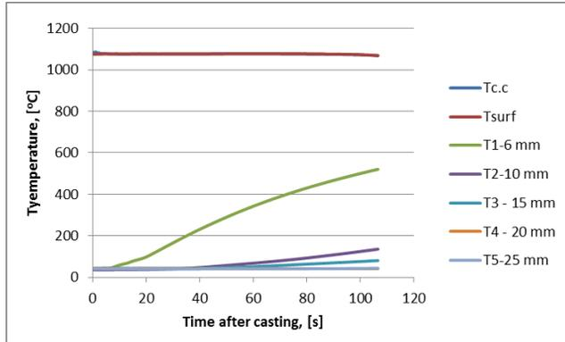
Fig. 3. Temperature field of the examined system. Tc.c is temperature measured in the centre of the plate-casting; Tsurf is temperature of the mould inner surface; T1 to T6 are temperatures measured inside the mould body on different distances from the inner surface
