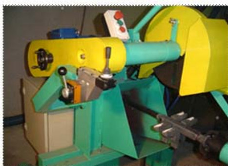
Fig. 2. Abrasive cut-off machine- general view
