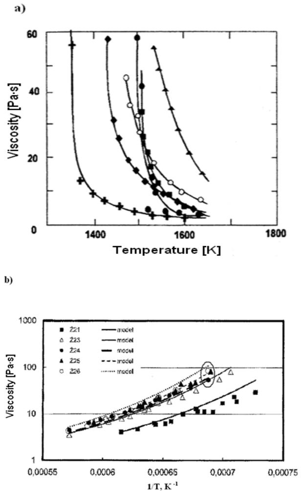
Fig. 1. a) Slag viscosity changes with temperature b) slag viscosity change at a given temperature at the various configurations [16, 18]
