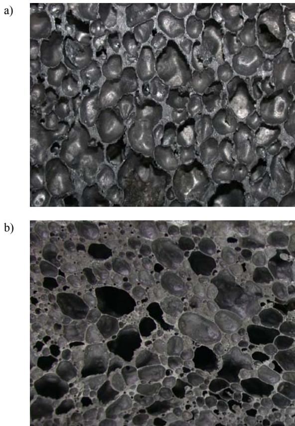
Fig. 3. Foam cross-sections: commercial foam (a) made at the Maritime University (b)
