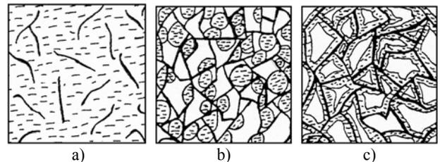
Fig. 2. Suspension structure: a – with continuous liquid phase, b – with discontinuous liquid phase which poorly wetting the solid phase, c – with discontinuous liquid phase well wetting the solid phase [5]
