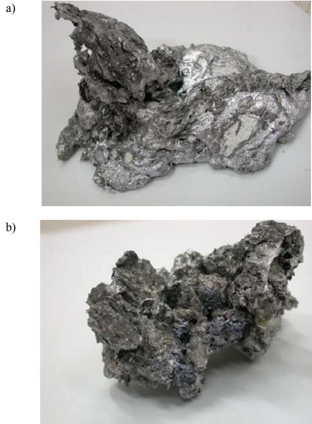
Fig. 4. Products of molten foam: commercial (a) and foam made at the Maritime University (b)
