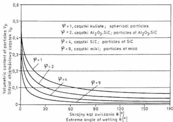
Fig. 1. Boundary volumetric content of solid particles in a continuous suspension in relation to the angle of wetting and shape coefficient [3]
