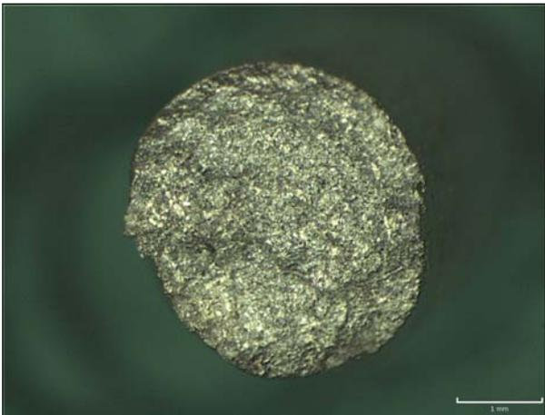
Fig. 11. Macrostructure of tested sample, 6 mm/min, 200°C
