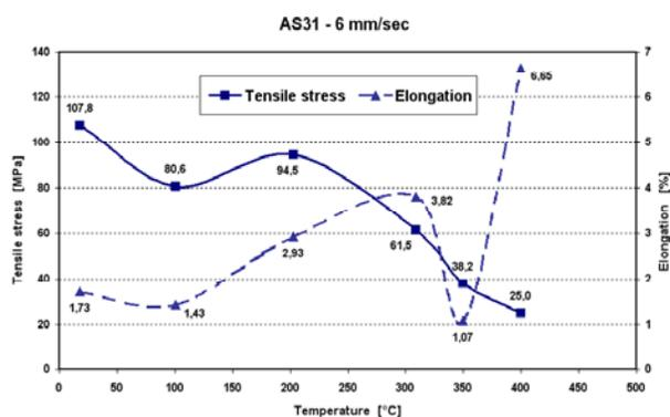
Fig. 4. Tensile stress, elongation – alloy temperature relation shown in graph; AS31
