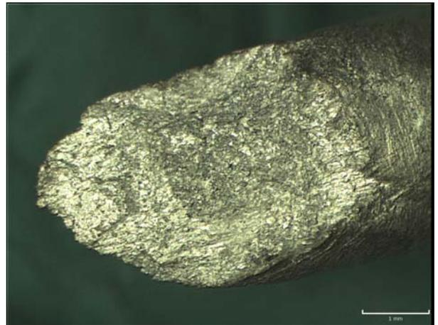
Fig. 12. Macrostructure of tested sample, 6 mm/min, 300°C
