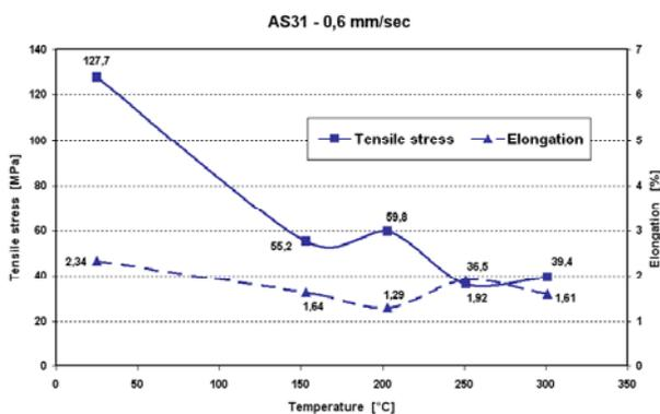
Fig. 6. Tensile stress, elongation – alloy temperature relation shown in graph; AS31
