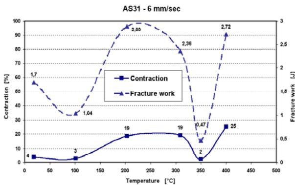
Fig. 5. Contraction, fracture work – alloy temperature relation shown in graph; AS31
