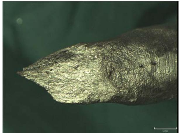
Fig. 14. Macrostructure of tested sample, 6 mm/min, 400°C
