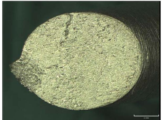
Fig. 13. Macrostructure of tested sample, 6 mm/min, 350°C
