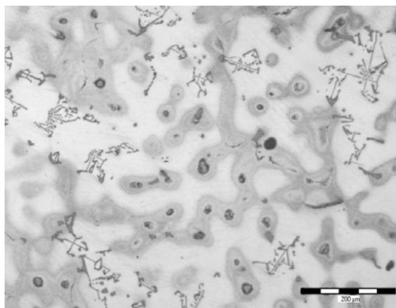
Fig. 2. Microstructure of source material – AS31
