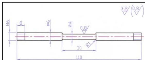
Fig. 1. Drawing of the test sample used in rupture tests
