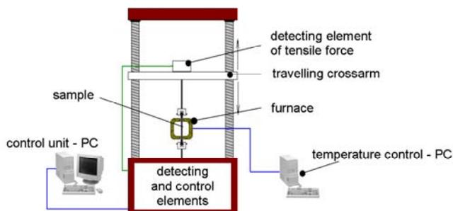
Fig. 3. Experimental set for measurement of solid and plastic qualities of ferrous materials treated in high temperatures
