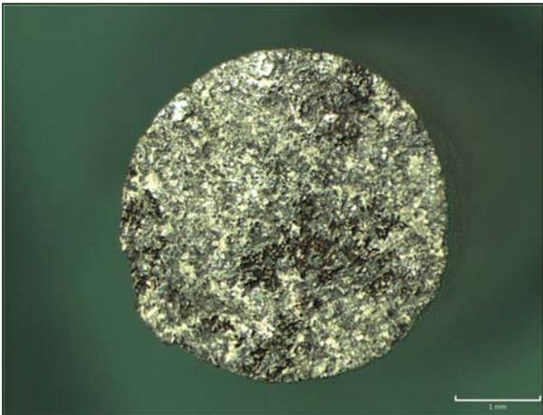
Fig. 9. Macrostructure of tested sample, 6 mm/min, 18°C
