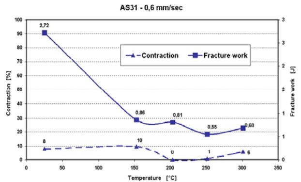
Fig. 7. Contraction, fracture work – alloy temperature relation shown in graph; AS31
