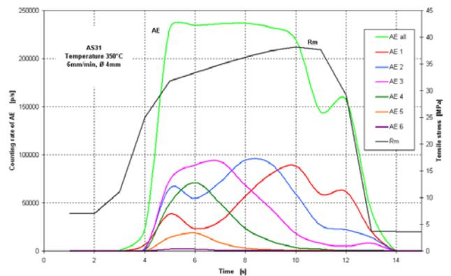
Fig. 8. Record of tensile stress with AE – 6mm/min, 350°C, AS31
