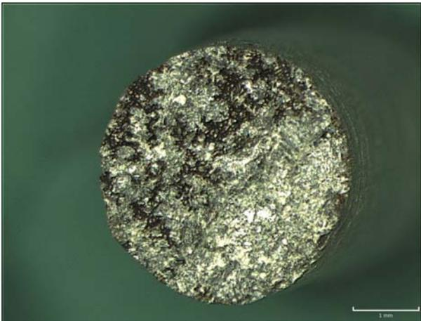
Fig. 10. Macrostructure of tested sample, 6 mm/min, 100°C
