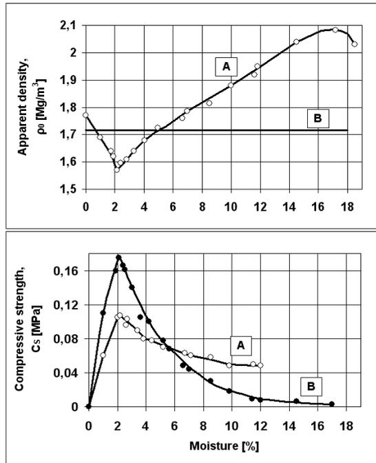
Fig. 1. Influence of moisture on compressive strength of a green sand, A – for continuous work of compacting the sample, B – for constant apparent density,  $\rho_0=1,715$  [Mg/m<sup>3</sup>] (prepared on the basis of [1])
