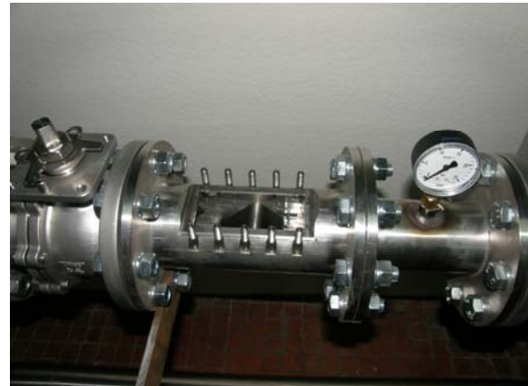
Fig. 3. A view of the cavitation tunnel chamber of the flow stand used in the present work
