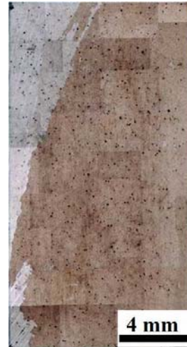
Fig. 9. Microstructure of the TZCC Cu-4.7 wt. % Sn alloy
