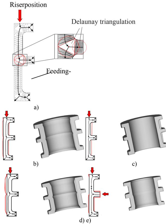
Fig. 4. Design by the cross section method
