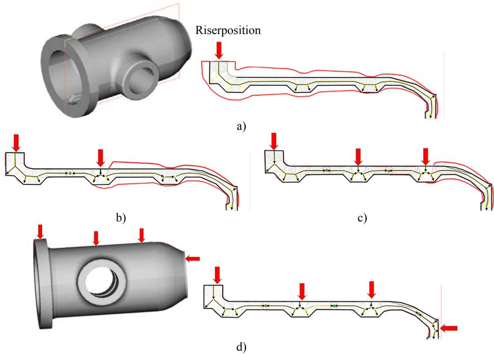
Fig. 6. Determination of a feeding system for the casting by the application of the module "CastDesigner"
