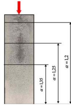
Fig. 1. The density standard for a casting of steel 35 L (GS-52) produced in sand mould
