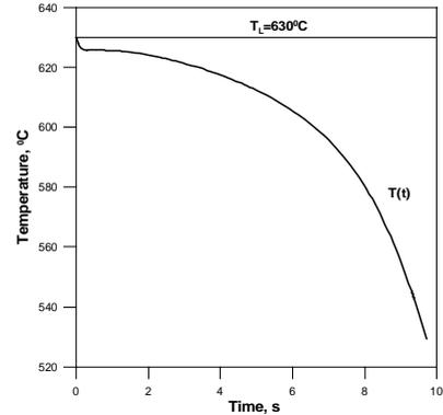
Fig. 3. The solidification curve of the model alloy
