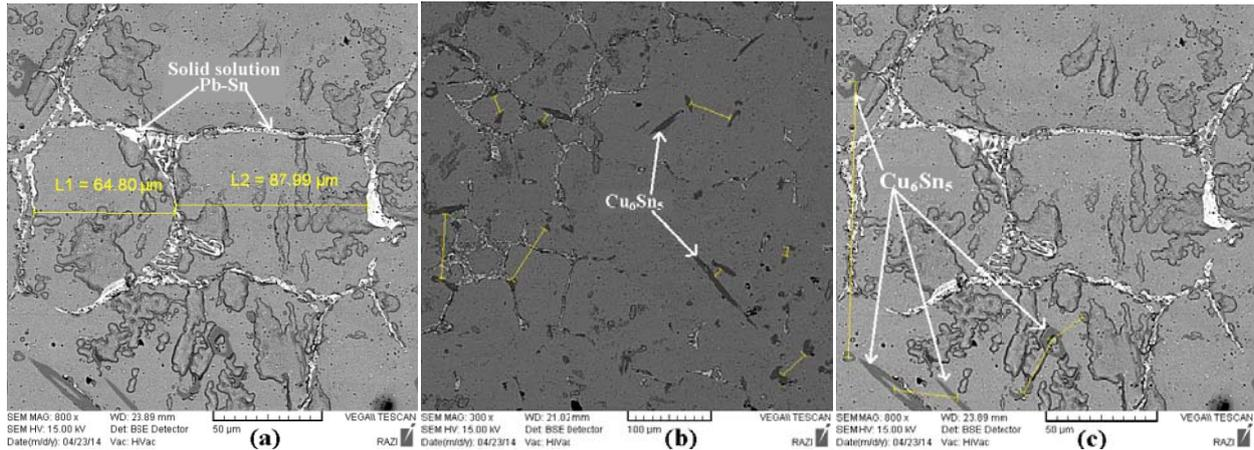
Fig. 5. SEM images (a) Average distance of solid solution of lead-tin (white continuous phase) from each other in the middle of thickness of product (b) Average distance of  $\text{Cu}_6\text{Sn}_5$  (dark gray needle shaped phase) particles in the outer surface of the product, (c) Average distance of  $\text{Cu}_6\text{Sn}_5$  particles in the middle of thickness of the product
