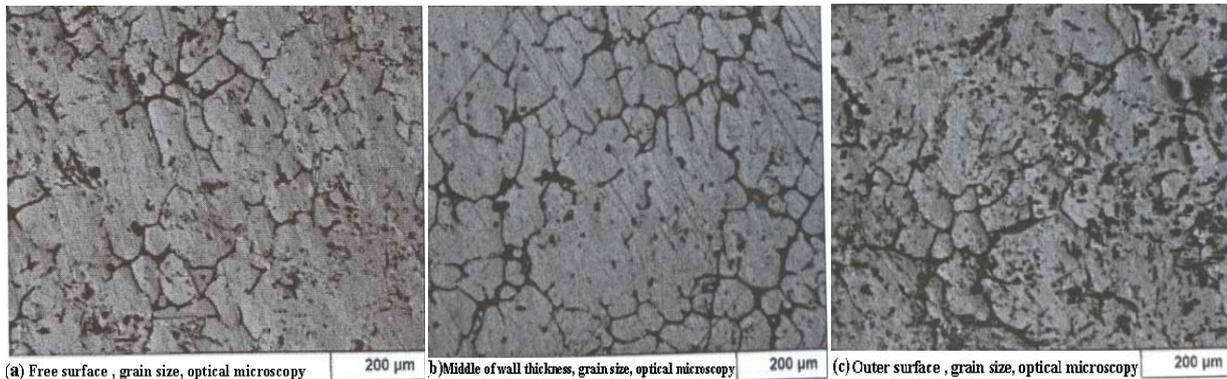
Fig. 4. Optical microscope, etching solution Nital 2%
