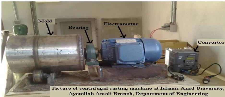
Fig. 3. Components of a centrifugal casting machine
