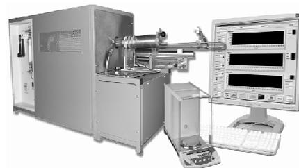
Fig. 1. Analyzer for determination of the lustrous and amorphous carbon in materials used as additives to the foundry moulds
