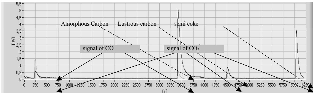
Fig. 2. Exemplary process of the pyrolytic carbon determination (fraction of the lustrous and amorphous carbon) and semicoke for the standard sample – tetraphenylsilane
