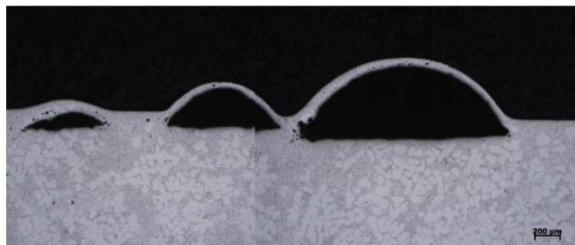
Fig. 3. Structure of the casting surface through the defects, 25x
