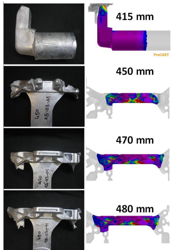
Fig. 8. Stop tests and simulation of the filling of the mold in selected positions of the piston
