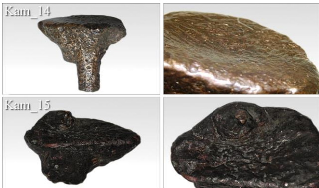
Fig. 5. The macrostructures of the main runners
