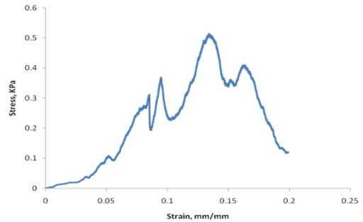
Fig. 2. Stress-strain curve at 18% clay content
