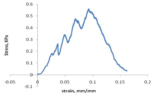
Fig. 3. Stress-strain curve at 22% clay content
