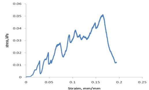
Fig. 5. Stress-strain curve at 30% clay content
