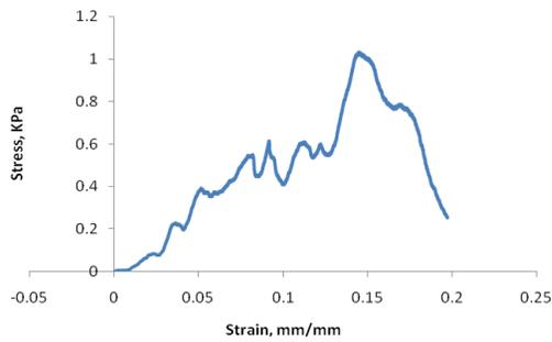
Fig. 6. Stress-strain curve at 32% clay content
