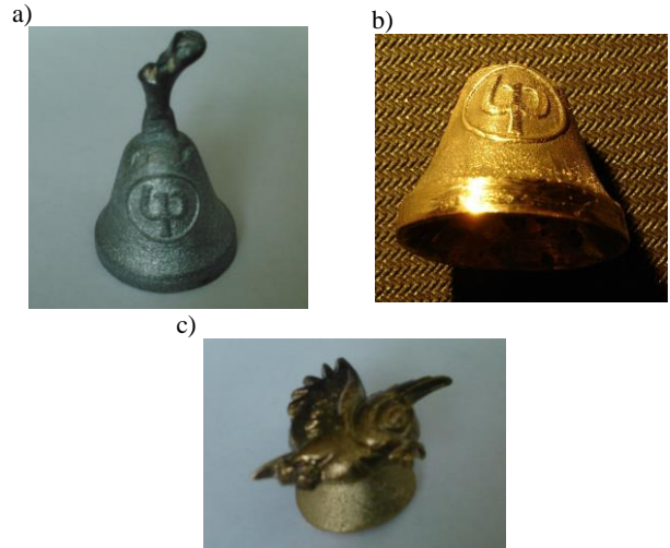
Fig. 7. Castings after knocking out and cleaning: a) ZnAl15, b) CuSn10Pb10, c) CuZn37
