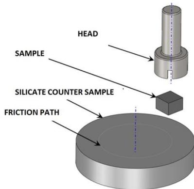
Fig. 5. Diagram of the steel and silicate counter-sample
