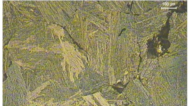
Fig. 2. Columnar and equiaxed grains, together, in the CET – zone, that is in the columnar into equiaxed transition zone
